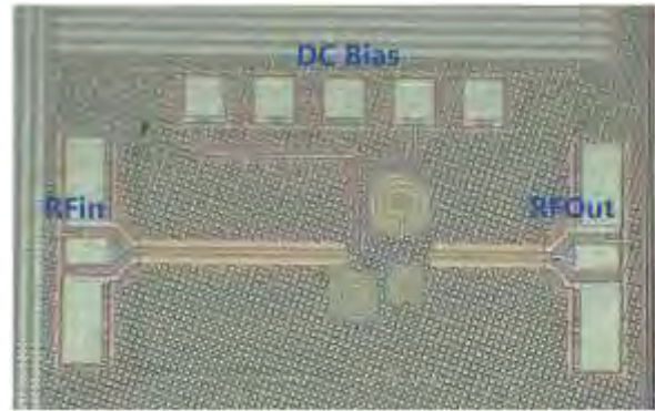
Figure 2. Layout and Chip photograph of the fabricated LNA.
